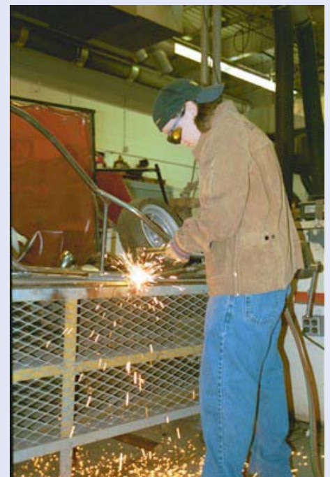
Amber is using an Oxy Acetylene Torch to cut metal in WTCC's Metal Trades/Motorsports Fabrication Classroom.
